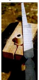
Wayne started the meeting in earnest with a show-and-tell of his method of putting a copper ferrule on a guardless knife. Here's my summary of the process - we'll hope I've got it about right! He takes a section of copper pipe and shapes it on a tapered mandrel that is the proper size for the handle material. The idea is to wedge the ferrule onto the handle, the compression adds to the strength of the handle. Wayne's mandrel is something he made
