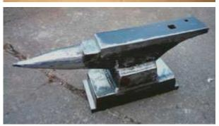
if I can get any weld done properly so I'm impressed. Keith beveled the edge on both the base and the anvil top to make a grove weld for better strength - and the anvil rings true!
