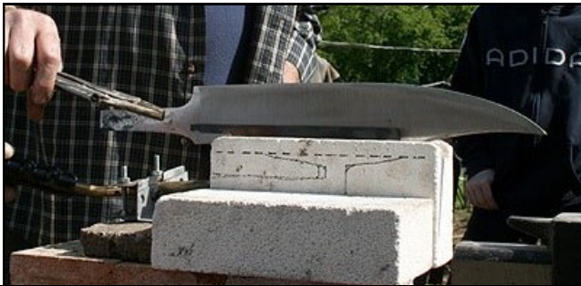
The soft back tempering gizmo is being heated as the blade is worked back and forth. More details on this at the meeting on Thursday evening.
