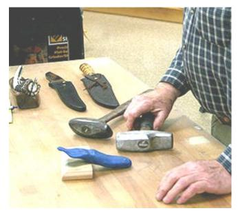
with a radiused edge to show how to move steel quickly in only one direction by holding the "steel" on the radiused edge at a slight angle and striking it so that the line of the peen in the hammer matches the line of the radiused edge of the anvil:
