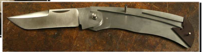
And here's the way the blade, spring lock, and back spacer fit onto the liner:
