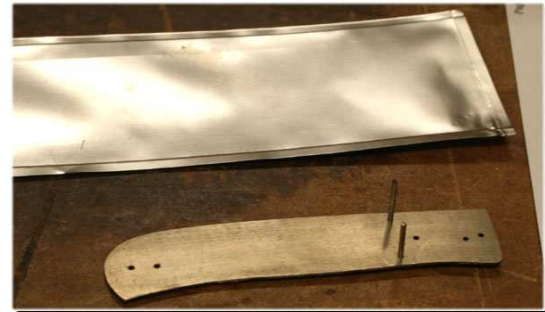
And one of the templates Jess showed us... along with the stainless steel bag he uses for heat treatment.
