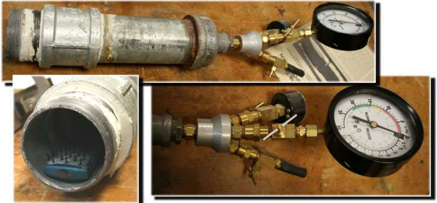
Here's a closeup of the fittings: the bottom line gets hooked to vacuum or pressure. The top two are pressure and vacuum gages. All three have shutoff valves so that the appropriate gage can be "on" and to hook up to pressure or vacuum.
