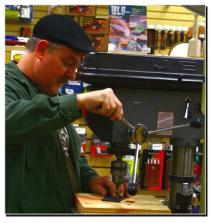
style sheath Jeff drills the 1<sup>st</sup> rivet hole about 1/4" down from the blade heel and 1/4" forward of the end of the handle. Decide how many rivets you want and drill the rest of the holes so that they are evenly spaced out to the point. Run the drill *very* slowly.
