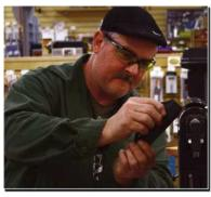
with the knife in it and the knife will not shake out. On the other hand you want the knife to be loose enough in the sheath that you can deploy it with two fingers. Getting the sheath grip "just right" can be achieved through both the final outline of the sheath, and if necessary using a heat gun to soften and reshape the throat of the sheath.
