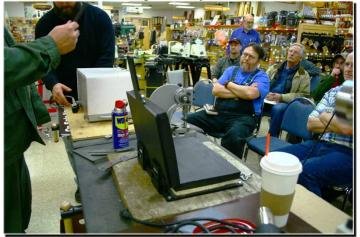
A toaster oven (white, at the far end) – a Kydex press (black, foreground) – a drill press, bandsaw, belt grinder, and a rivet press (gray – between the oven and the Kydex press in the above photo). Sure – you can set the rivets by hand, but if you do any quantity the rivet press is a sanity-saver.
