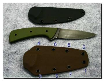
If you need to re-heat and re-form the sheath after the first rivets are set, do *not* put it back in the oven as the Kydex will pull away from the rivets – use a heat gun to re-mold portions of the sheath as needed.
