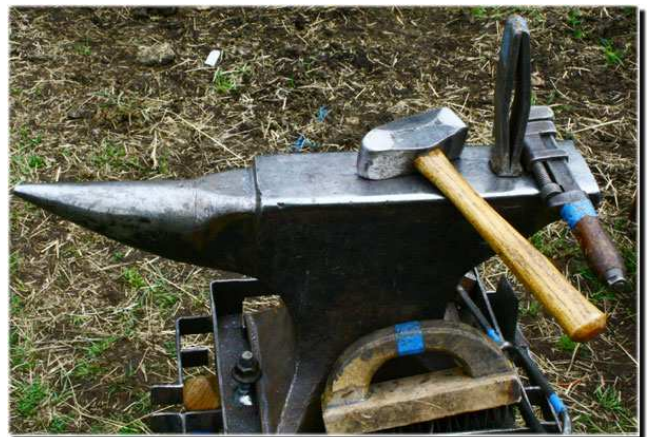
Marty Brandt's anvil – note the straightening jig in the hardy hole:
