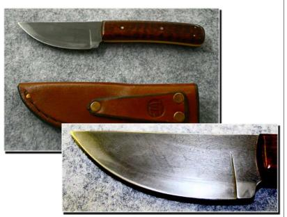
Wayne was asked how he prepares cable for forge welding. He responded that he unbundles the cables down to the individual strands, cleans them, rebundles them and uses an Oxy/Acetylene torch to weld the ends together. He heats up the reassembled cable and twists it up tight. He puts together multiple cables worth – up to thousands of strands – so that you have enough material for a knife without making the individual strands too thin – so it still has a pleasing pattern in the finished blade.
