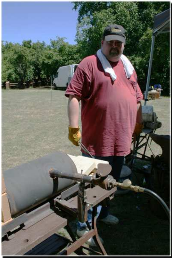
And here's Walter Hardcastle with his forge. Note the homemade venturi he and Dave Rider put together.
