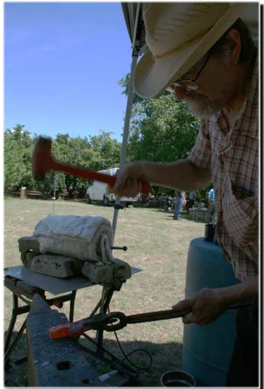
And our host's coil-o-Kaowool forge (around a ceramic pipe, I think).
