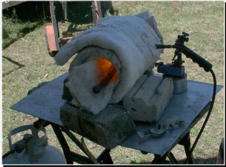
And our host's coil-o-Kaowool forge (around a ceramic pipe, I think).
