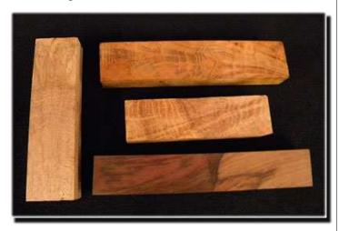
Typically, when a piece of wood is cut directly in line with the end grain, the sides of the scales or handle will be very plain. When the same piece of wood is cut at slight diagonal to the grain lengthwise, the side will show a banded "U" or "V" pattern:
