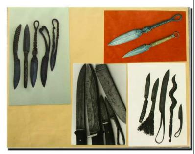
This just reinforced what Lynn had gotten from a blacksmithing class – that whenever you finish forging a piece of steel you do two or three normalizing passes on it to refine the grain size, remove internal stresses, etc. Lynn noted that to do normalizing you bring the steel up to just above where a magnet stops sticking to it and let it cool back to black in still air. If you harden and break the steel after normalizing, the grain you want to see is silky smooth, not course and grainy.
