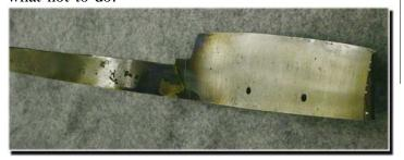
The knife re-tapers right at the tang – which failed the bend test. After it broke at the tang, Wayne brazed it back together to see what the rest of the blade was made of. On breaking the tip, you can see course grain structure – like beach sand. Not acceptable.
