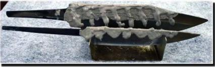
"You have to be sure that the claying is 100% dry – otherwise it's going to bubble up, it's going to blow off, it's going to do many strange and ugly things." He lets the clay dry for several days. If you try to heat it to dry it the clay will bubble up. When it is truly dry it becomes really hard.
