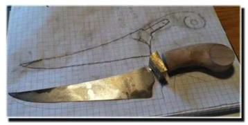
So: toss one in the "oops" drawer and do-over. I'm anxious to try out this chef's knife design – so I have a replacement blade in progress. I'm making the blade from a billet of cable "Damascus" I forged last Fall.
