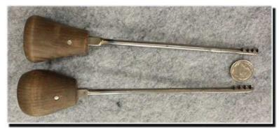
Mike took an old used-up file, ground the teeth off, cut strips out of it, annealed it, cut teeth in it, heat treated it, and put handles on it.
