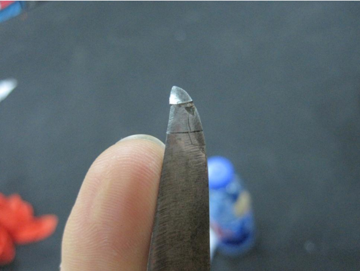
High carbon hard face cracks, body does not.
