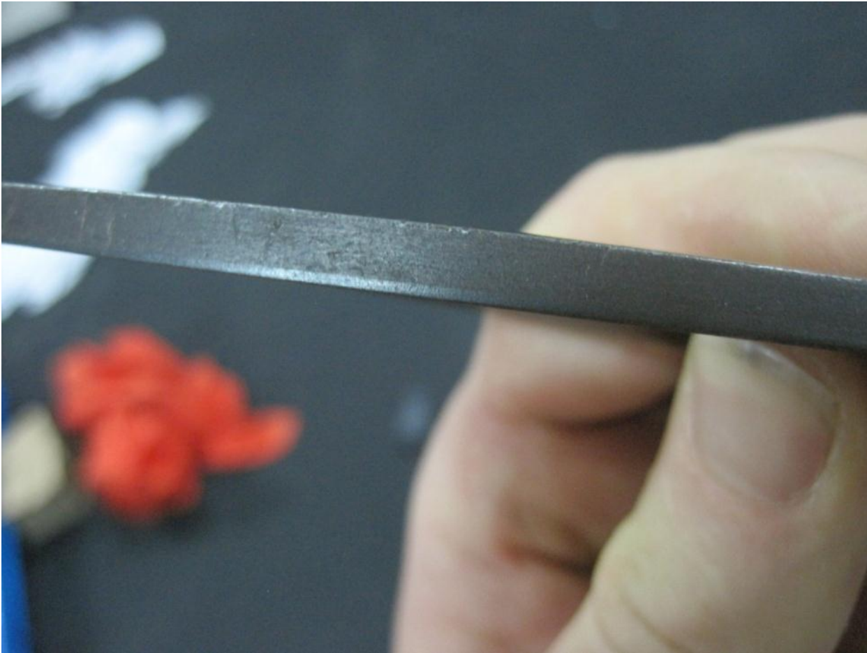
High carbon cutting face does not rust in the same way as the rest of the scissors. Note the bright line 1/16^{\text{th}} thick.
