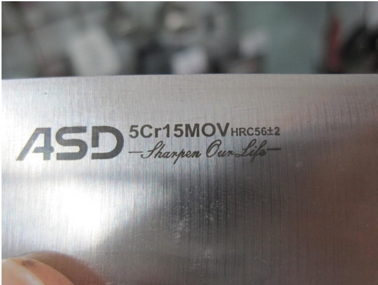
A knife in a store in china with alloy and hardness noted. First time I'd seen this.
