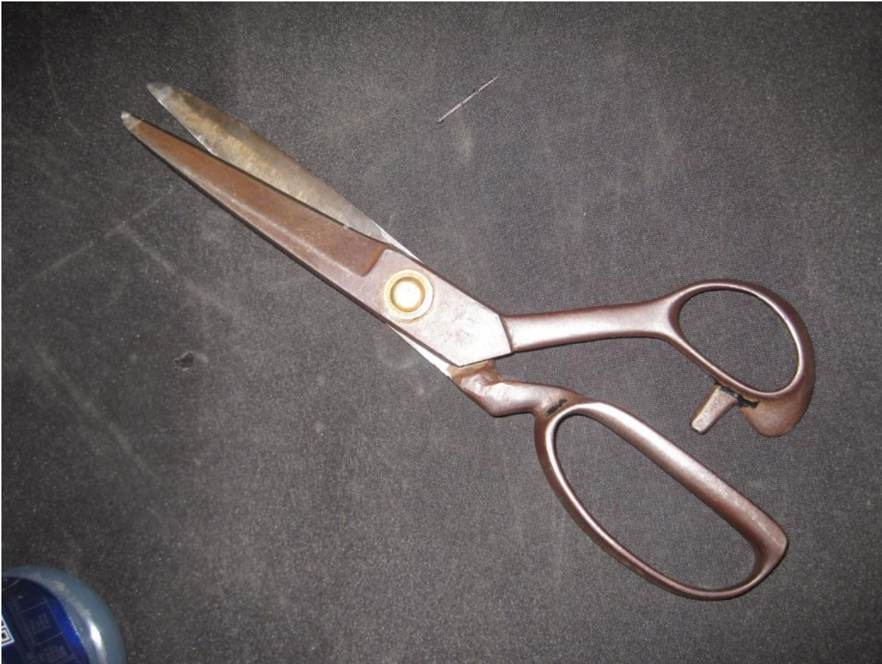
Old tailoring scissors, laminated blade faces.
