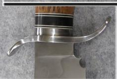
To secure the butt cap mike brazed a threaded sleeve on the tang and used a bolt through the butt cap to tighten it all up. He did file work on the bolt head.
