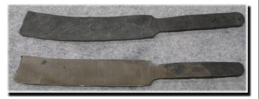
He got a good amount of advice on how to proceed with these blades – as well as on forging and grinding in general. How to pre-form the steel before shaping the knife. How forging the main bevel makes the tip swoop up. How to correct that with a schwocking stick.
