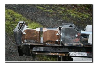
I had to true up the rail faces. And I had to add some brass bushings to the ram head to take some slop out of the action. And it's still kind of sloppy... but hey! I've got a wood splitter and a forge press!
