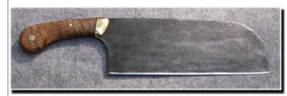
I put a slight reverse distal taper on it to have a little more weight out at the end of the blade for chopping. After tempering it's about a 60 Rockwell. I'll put a longer handle on the next one I make.
