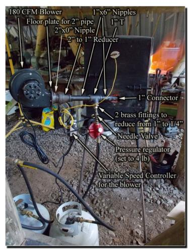
I got all the black pipe from a hardware store plumbing department. DO NOT USE GALVANIZED PIPE – the zinc will vaporize at high heat and can make you sick. The "bell" on the end of the burner is just a 1" connector. I didn't smooth it out or anything.
