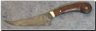
This kitchen utility knife's 5" blade is of 1095/15N20 Damascus from a 700 layer billet. It's just over 9" overall. I made the handle longer than the prototype based on our daily use of the prototype knives. The bolster is brass with red and black spacers. The handle is bubinga finished in a mix of bee's wax, carnauba wax, and food grade mineral oil. This mix is food safe and stood up well in my testing and in daily kitchen usage. That's a Sally Martin mosaic pin.
