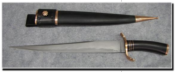
Evan heat treated the hunter "and now the file won't work on it!" So he's looking at hand work to finish the geometry. Jove Lachman-Curl suggested using a 2x72 belt wrapped around a piece of 1x2 – as a better "paper" than generally available – until you can buy or make a belt grinder. Jove noted that
