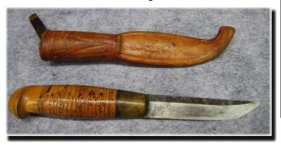
As with most scandi knives, the primary bevel of the knife goes all the way to the edge. The knife is sharpened by laying the entire face of the blade on the sharpening stone, so that the main bevel continues to the edge with no secondary grind.
