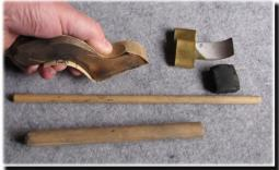
I also showed the tools I use to finish up the scroll I use on the end of these kitchen knife handles: a small straight chisel and a riffler...
