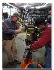
And David had a project of his own: turning a heavy chunk of steel angle into a mounting bracket for a post vice. With Lynn Moore as striker they punched then drifted three holes that will bolt into the post vice stand. David plans to cut lobes around the two U bolt holes on the vertical side of the piece and just in general give it his artistic touches. A fun time was had!
