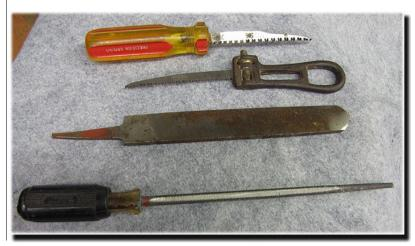
Martin noted that you can remove older screwdriver handles by putting them in warm water, put the shaft in a vice, then pry-bar the handle off.
