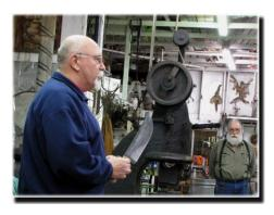
Well, I took a small piece – 3/8" thick by 1" and twisted it – forging it as I twisted it and forged it at high temperature. Turned out really nice..." except that it was slightly warped
