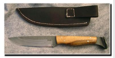
Frank wanted to try making a blacksmith's knife. And after making this one with flat stock and dealing with the 90° change in 1084 "flat" between the blade and handle he recommends starting with ROUND stock next time!
