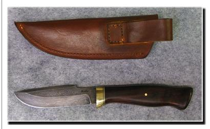
"I just about finished up two cable Damascus knives" [except for additional coats of finish on the handles]. The light handled one is from 1" cable, the dark handled one is 7/8" cable.
