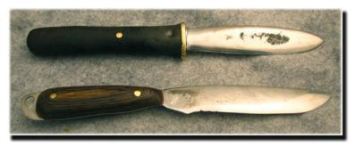
Frank and Lynn noted that even if the RR spike is stamped "HC" for "High Carbon" it's not "high carbon" in the knifemaking world. At most it would be 0.35-0.4% carbon whereas 0.5% carbon is the low end for what knifemakers buy from the mill – and might not refer to steel as "high carbon" until you get to at least 0.8% carbon. You can still make a good
