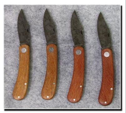
The wood is finished in by sealing in 4 coats of cyanoacrylate (Superglue), sanded smooth, then 3 or 4 coats of Renaissance Wax.
