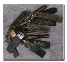
spark test unknown materials and come up with a pretty close guess as to what you've got and about how much carbon it has." He started out doing spark testing for welding with recycled steel so he'd know if he was trying to weld with high carbon steel or not. High carbon having more of a tendency to crack at the weld if not cooled slowly.
