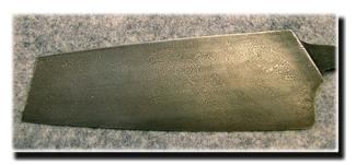
There was a lot of discussion about my heat treat process – and alternatives like quenching with aluminum plates prior to grinding in the bevels, etc. and just in general, quenching full thickness then grinding the hardened steel. If you do that, Craig Morgan recommends knocking the edge off the profiled blank before hardening – because if you grind hardened steel with a sharp, square, edge it will peel grit off the belt.
