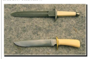
Craig responded to questions by describing some of the working processes. "You have to come up with different ways to hold things... the guard sits on to end of my finger!" He started with a round hole in the guard – filed it rectangular with a tapered square needle file and an OptiVISOR. Once he had the hole made he used a Dremel mandrel – with the screw through the guard – to give him a handle on it.
