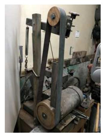
Wayne told me that a two wheel grinder has the most torque. Each additional wheel added to the system reduces the grinder's efficiency. By bolting the frame together rather than welding (not one of my specialties at that time), the frame can be adjusted when it's not aligned.
