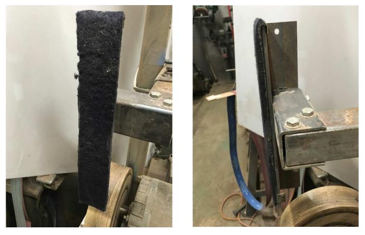
Another different platen attachment is a felt platen. Wayne used a harder felt than I had, but mine seems to work.
