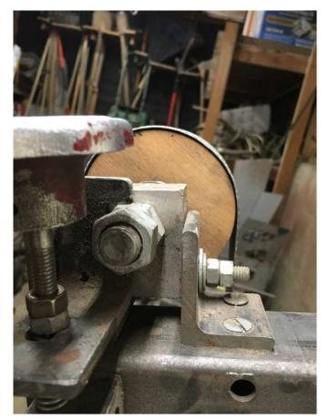
Double nut the end of the 5/8" bolt on the back side of the aluminum block.
