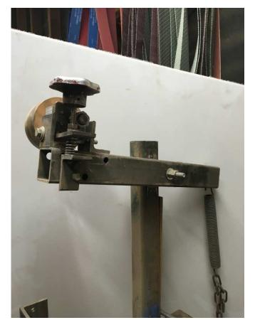
This whole idler/tracking mess is mounted on top of the top pivot arm that is attached to the mast. A strong spring on the end of the top pivot arm gives the tension needed to make the belt keep traction on the drive wheel.
