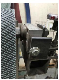
I tried a couple different tracking adjustments that worked (poorly). This system works well.
