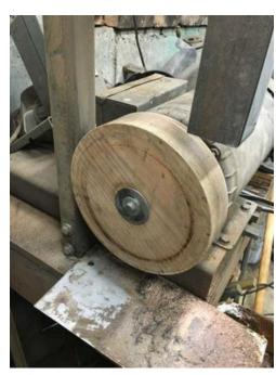
on the end of the shaft. This kept the wheel from flying off, but not wandering. I drilled and tapped the wheel opposite the keyway. Inserting a long alan set screw into the hole and tightening it down helped, but still didn't stop the wandering until I drilled a recess into the motor shaft for the set screw to tighten into.
