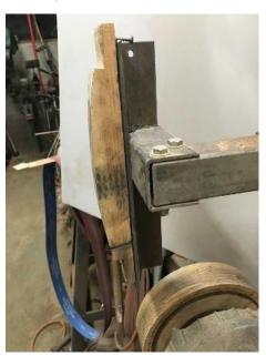
I started out with a 2X4 on my band saw to rough out the shape. I used an adjustable auto body filing tool as a template to set the curve. This is a tool with handles and a plate that has a turn buckle on the back to create a wide variety of curves in auto body repair.
