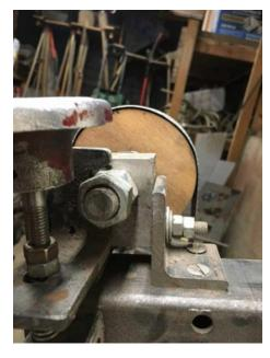
turned, the whole aluminum block with the idler/tracking wheel pivots up and down. When the belt is running, this pivoting of the idler/tracking wheel makes the belt move side to side over the platen and drive wheel.
