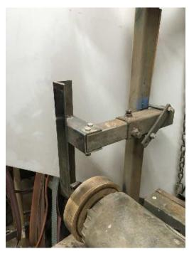
A "U bolt" attached the receiver for the platen. I found that I needed to adjust the receiver tube to align the platen. A thin wedge of wood on the back side of the mast took care of the problem.
