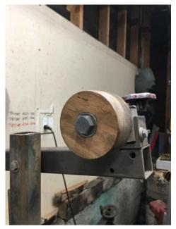
The idler/tracking wheel is a different story. 2" thick oak, turned to 4" diameter was a good start. For the 2"X72" grinding belt to track straight and adjust from side to side, the idler/tracking wheel has to be slightly crowned. Since it was still on the wood lathe, working a slight crown with a file was easy.
