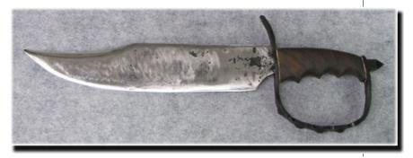
The D guard is forged from flat stock – using swages and grinding to get the knobs and valleys.
