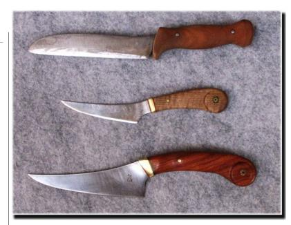
I didn't have a belt grinder yet when I made the old ugly one at top. I'd taken a hunk of modeling clay and squeezed it in my fist as a mock-up for the contours of the handle. It was satisfying to have a knife handle that really fit my hand. I've since gone for a more stylized handle shape – but I've kept some of the contouring of that original handle design so that I'm still still happy with how it feels to pick up my knives. And they look a little better IMHO.
