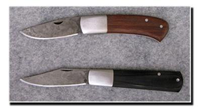
The liners and bolsters are 410 stainless. The springs are O-1 tempered way back.
