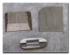
You can see the grain a little in these lightly etched and bent samples.
