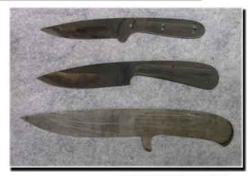
**ERIK LAND** took the floor next, passing around the last two folders he is completing using high carbon steel. One has stabilized sycamore scales – the other is in buckeye burl. They both have "French Etch" aka mustard finish on the blades.
