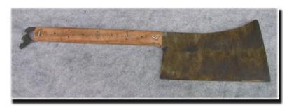
Next Lynn passed around a number of knives-inprogress mostly made from the bandsaw steel Dennis provided. One has a handle made with sycamore that Frank Bobbio stabilized.
