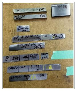
side. So while my portable tester always hits it on the money on the thick flat reference block – it's not reliable on thin beveled blades – at least not how I've been using it. I'll have to see if I can change methods to get more accurate results.
