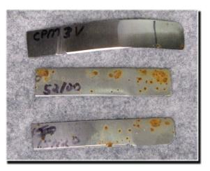
As you can see, the 3V did very well. The 52100 rusted a little more than the 15N20, but not that much more. The 3V sample is bent because Frank had done a test heat treat on it that got it to 59 HRc – bent it to 100-110° without breaking – and it came back to this maybe 60° bend.
