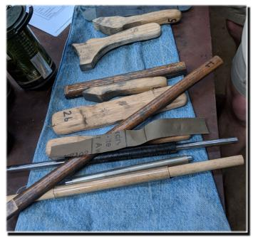
Gluing on a layer of leather or soft rubber will give sanding for an eased edge. Gasket material or mild steel facing gives you a firmer or sharper edge to work flat or corner areas.
