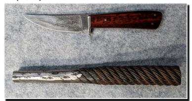
Dennis has handed off some of the cable to me-I will quench test a piece and if it shatters nicely (is hardenable in water) I'll chop it up and bring it to the hammer in.  $\sim$  Michael Kemp
