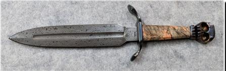
Somebody asked Frank how he did the fuller. "To start with I ran a 3/8" ball in the milling machine..." and then went to hand grind it with a 5/8" small wheel – but the wheel kept catching the blade. To clean up the wobble he used a diamond wheel on his flex shaft tool – and using his finger on the edge as a guide he took 1/8" off the sides of the fuller. Then back to the grinder with a 1" wheel and used a slow speed to finish it up.
