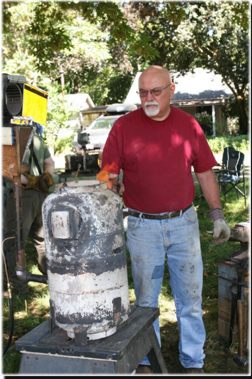
Mike Johnston and I were the first ones on site. Here's Mike tending his propane "bird cage" forge – heating some cable to make cable Damascus.
