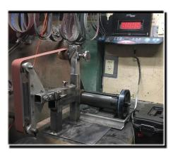
filed down to accept 1-3/4"x1-3/4"x.120" inserts. The outside of the 1-3/4" has to be draw filed or belt sanded enough to slide inside the 2" receivers. Mike
