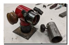
The inner tube pictured above is set up with leather insert so that you can clamp a blade with a finished handle without marking it up.
