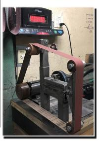
noted that he had to true up the inside of the 2" tubes with a file after welding everything. The bottom of the tracking tube is welded shut and a valve spring dropped in for tension. The mount for rollers and platen is 1/2" aluminum plate. The base is 1/4" plate.
