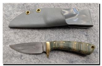
The home-made "micarta" handle is 12 layers of a denim material all aligned to give a solid block effect to the fabric pattern.
