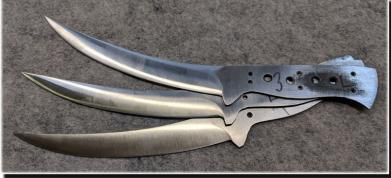
Mike hand-forged the next pass-around out of pickup coil spring. The handle is ziricote with brass guard and Sally Martin mosaic pin.
