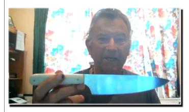
"I've been using it in the kitchen... just to give it a try... that CPM 154 is HARD STUFF!" Lynn heat treated the blade between profiling and grinding – sounds like the grinding took a long long time. "I don't think I'll do that again."
