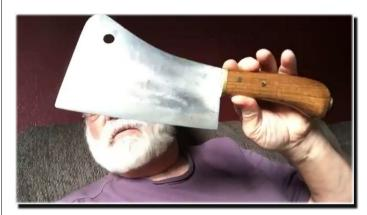
He knew this would get heavy use (it's been used to butcher moose) so he has both pins and the button butt cap. He threaded holes in the tang and used brass bolts for the pins. "I wasn't thrilled with the result – there were some little voids that I filled with finish.
