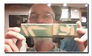
It's a piece of 2" PVC pipe that is heated and pressed flat (with room for the blade). Brome leaves an extension of one side of the pipe that he then heats that and wraps it around for a belt clip.
