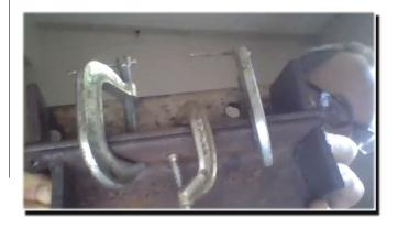
I noted that one of the chef knives I made warped at the edge but not at the spine – and I used the in-thetempering-oven method with a broken tip from an old failed blade to put bending pressure on the edge but not on the spine.
