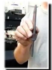
Frank noted that when he makes matching top & bottom dies for his press he will make the bottom die first. He assembles the top die parts on top of the bottom die and presses them in place and welds the top die together right in the press so that it is properly mated to the bottom die.
