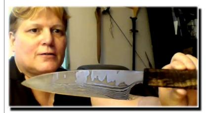
The waterfall/ocean billet at the edge is 15 layers, sideways. The cloud billet at the spine is basically san mai, although he used three layers of 15N20 on each side, 1080 in the middle.
