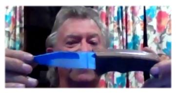
On the next work-in-process Lynn showed where the tang on a stainless knife broke during straightening after heat-treat. He silver braised it back together.
