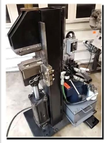
The void he mentions is hidden by the solid bottom die in this photo. Replace that with a die with punchthrough holes and your plugs will fall down and out the side of the ram
