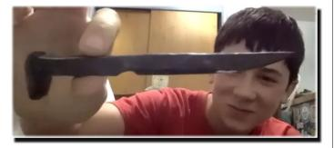
He mentioned that he was not able to get it to harden. RR spikes are *not* what a knifemaker calls high carbon, and will only harden using techniques that would shatter high carbon knife steels.
