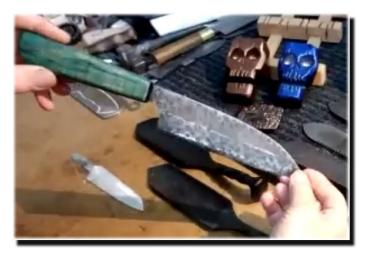
He's also worked up about 8 blades from AEB-L that are also for single bevel (chisel grind) kitchen knives.
