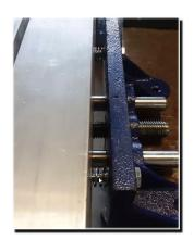
He also has made some quench/straightening plates out of 1-1/2 x 4 x 12 inch aluminum bar stock. He will experiment with plate quenching his Damascus. He bought a Harbor Freight bench vice which he fitted with bolts and springs to spring-load the plates so that they can adjust to any taper in a blade being straightened or plate quenched.
