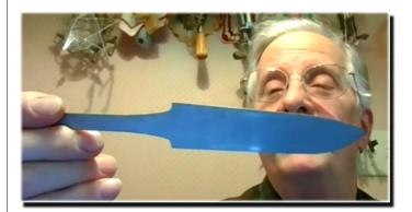
Martin described the explosive welding process. The layers are very clean when layered up. They put an explosive on the stack and when they set it off the force of the explosion drives out the oxygen between the layers and the heat and pressure fuses the layers.
