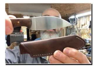
Brome talked about the trade-off of constructing a sheath with the belt loop integral to the pouch sheath but showing the rough flesh side – versus making a layered sheath with the back of the sheath having the grain side in, so that the integral belt loop presents the grain side. Wherever he does leave the flesh side out he coats it with tragacanth gum to smooth it down. He also uses that gum on exposed leather edges that he burnishes.
