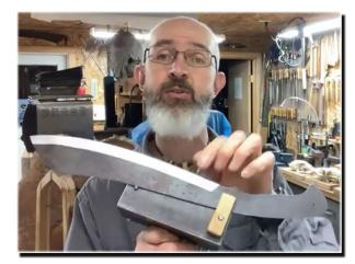
It's a big chunk of angle iron with two identical holes drilled in the face – one for a resting peg and the other for a clamp to hold the tang down and secure the knife. These can be reversed so that you can flip the knife around for grinding the far side. Before flipping the blade over Brome marks where the blade registers against the jig so that he can set it at the same depth/angle when it's flipped over.
