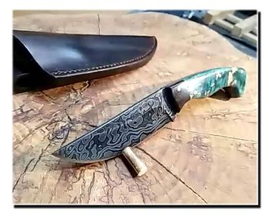
The handle is his own stabilized wood with a Super Glue finish. The blade is made from layers of 0.070" thick 15N20 and 0.035" thick used blades from home sawmill bandsaws. Those blades are sold in various grades. The ones that Frank came up with were the lowest grade but tested out at 64 HRc. So using this home sawmill bandsaw steel was one part of the experiment.
