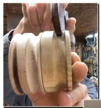
Brome has made a couple of burnishing wheels – hardwood disks with groves radii of 1/4", 3/8", 1/2" which he chucks up on his buffing wheel and runs against the leather edges to burnish them.
