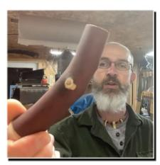
chunk for the handle of a harvesting knife, looking fully dried. Brome compares the bark to leather in that any marks you make on it while wet (intentionally or accidentally) will be there forever.
