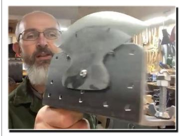
He noted that because of the curve of the blade, the angle of attack of the belt grinder changes as you go from the center to the two edges. So while he roughed in the bevel with the jig using a 36 grit belt, when he goes to finer grits he will lose the jig and true up the bevel by hand.
