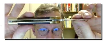
Back to the Sheffield knife, Edward will polish the inside of the liner and engrave his name there. He also plans to do file-work on the spine of the liners, and use a grinding stone on a Dremel for more "file-work" on the lock-bar.
