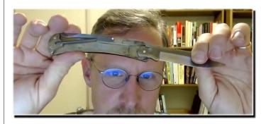
Here's the sacrificial knife that Edward uses to cut through the folder pins. It's an Ontario/Old Hickory kitchen knife. It's thin enough that he can get it between the bolster and the blade, then baton it through the pins.
