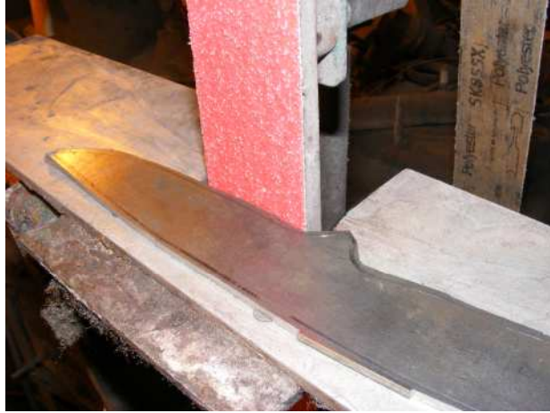
Working on profile refinement
