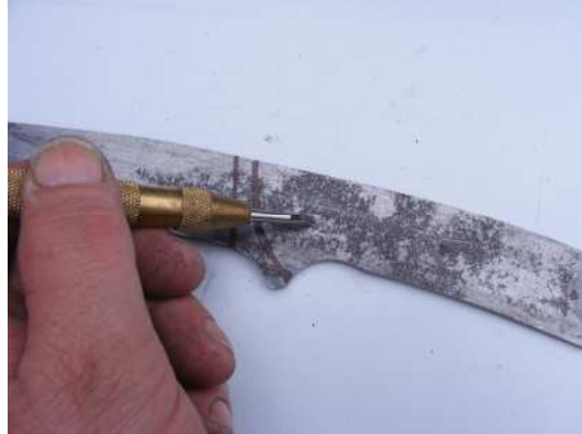
Using my punch tool to place divots in the handle for pre drilling
