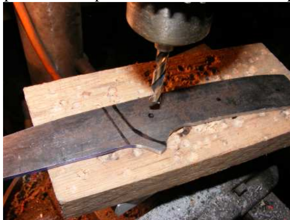
Aligning up the drill with the divot then drilling out the 1/4 inch holes
